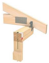
Pryda Screw used with standard MultiGrip secured to ribbon plate. 175mm screw installed through the top plate and ribbon plate.
