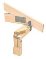
Pryda Screw used with Long MultiGrip secured to top plate. 135mm screw installed through top plate only.
